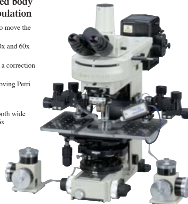
Configuration with Narishige micromanipulators and epi-fluorescence attachment
