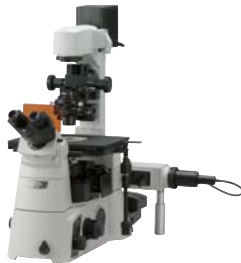
Ti-U configuration with epi-fluorescence illuminator
