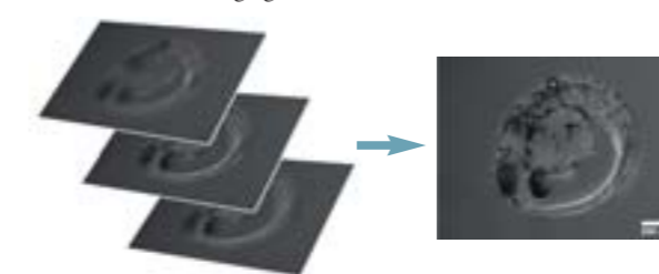
All-in-focus image created from a sequence of Z-stack images
