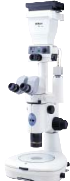
SMZ1500 configured with P-IBSD2 Beam Splitter D2, H-III-P Photomicrographic System, and CCTV camera
